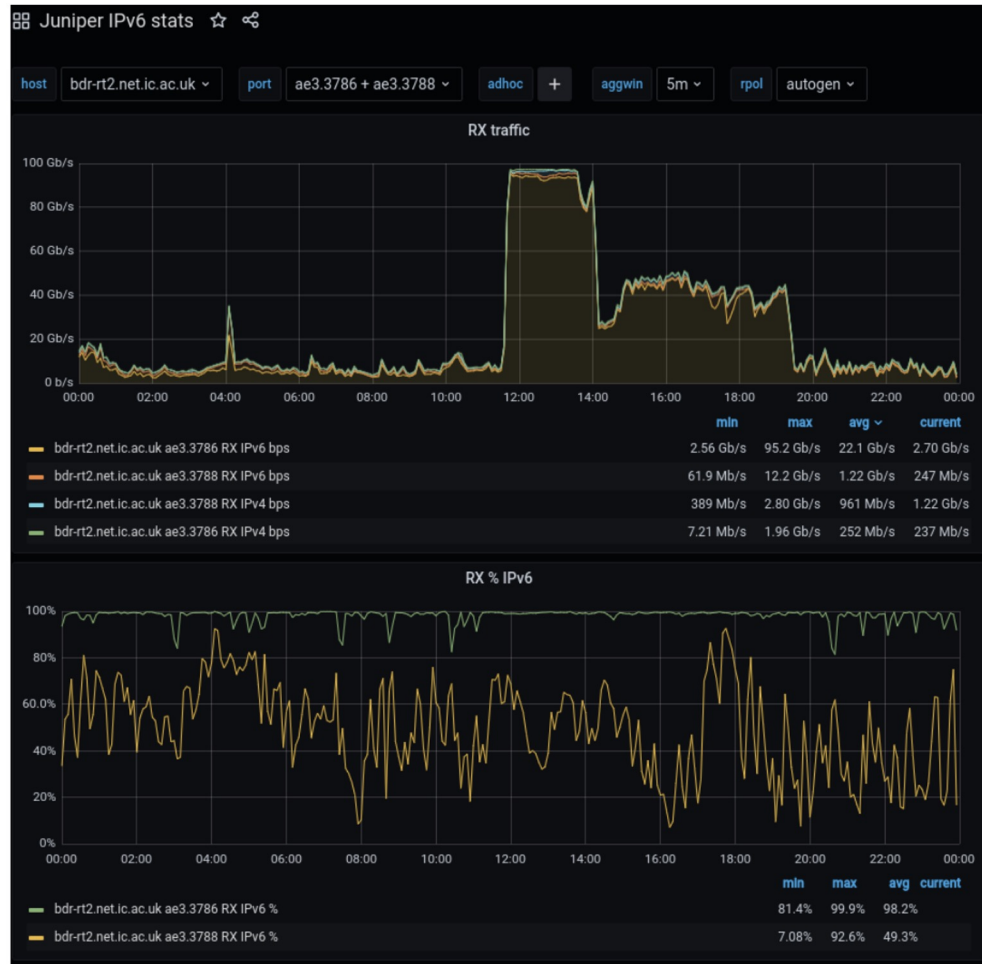
Figure 1 — Imperial monitoring shows the two-hour period where the 100G link was filled and where 100% of the LHCONE traffic was IPv6.
